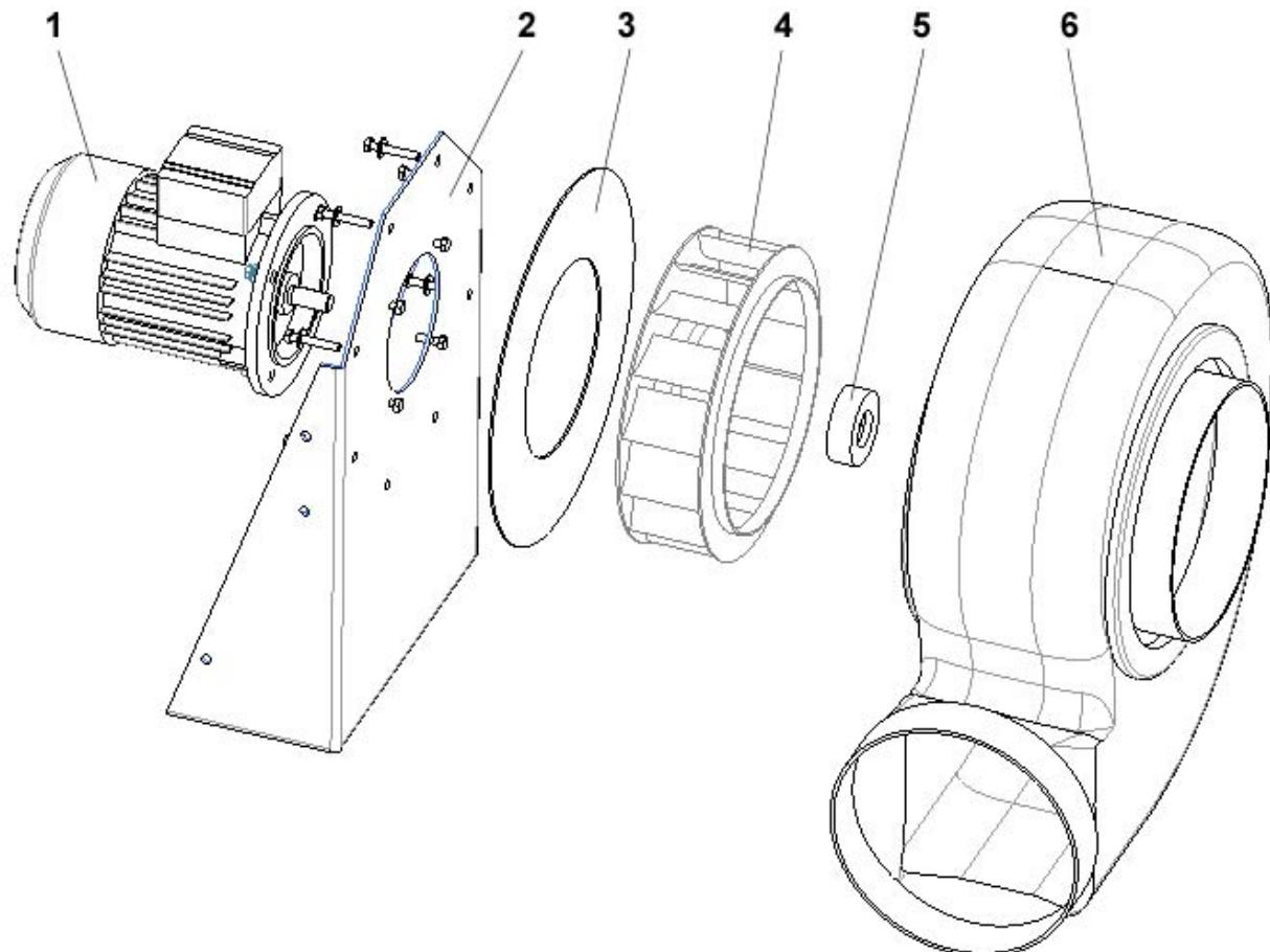
**1    MOTOR****2    MOTOR SUPPORT****3    DISK MOTOR SUPPORT****4    WHEEL****5    OGIVE****6    VOLUTE MOULDED**
